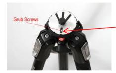
Using a small screw driver, there is a small security screw on the tripod head to lock in the clamp
