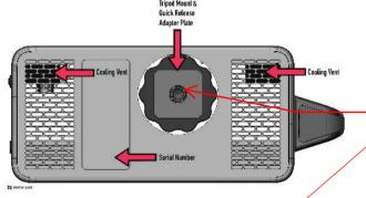
On the Pro 2 - Slide this plate into the clamp, and tighten the clamp head
